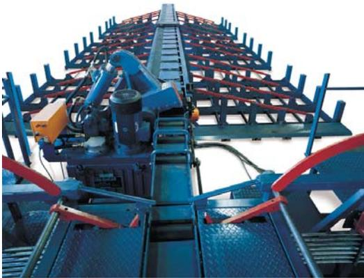
The system integrates the RSM 50.300 shear with conveyor width of 320mm. Option of single side or double side cut steel storage. The gauge table discharges the cut steel with pneumatically operated tilt action in both directions into 3, 4 or 5 storage bins per side. The conveyor rollers are 45 degree gravity coned to prevent steel running off the conveyor rollers.
